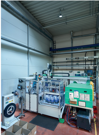
Fig. 2. Goerlich manufactures enclosures for vacuum sensors efficiently and flexibly with its compact turnkey system © Arburg
